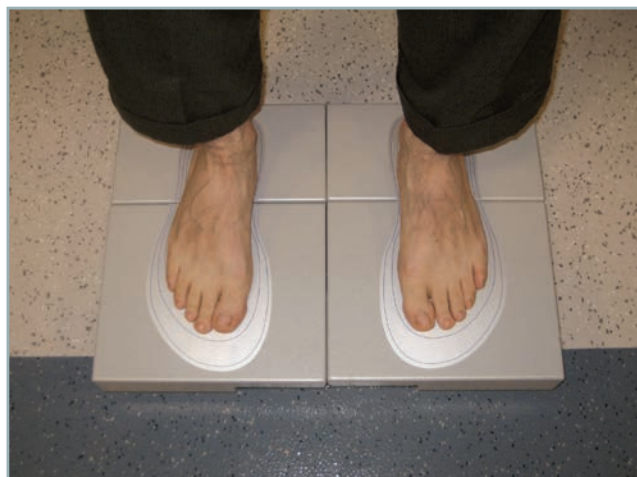
Figure 1. Quadruped scale with foot silhouette used to measure total weight and weight distribution through each lower extremity.
