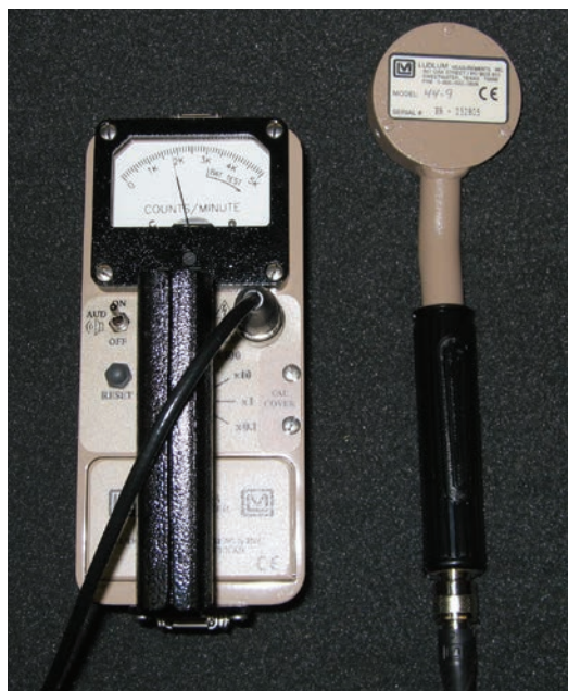
Figure 1. The contamination survey meter, or Geiger-Müller detector (often called a Geiger counter). Most often, the detector consists of a tube contained within a pancake probe (right). Although design and appearance vary according to manufacturer, Geiger-Müller detectors are able to read ionizations by means of an inert gas placed within the tube.
