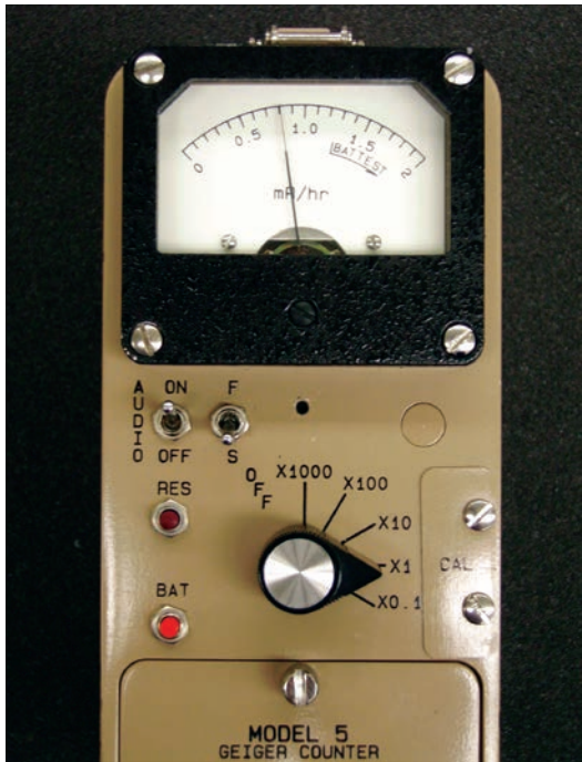
Figure 2. An analog display on a Geiger-Müller detector, with audio indicator and multiplier switch.
